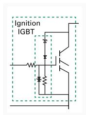
They provide protection against transient surges: load dump, ignition coil interruption and other switching spikes.
