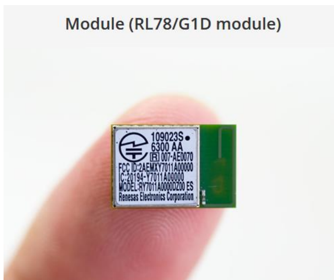
Figure 2. The RL78/G1D module incorporates an antenna and a RF circuit
