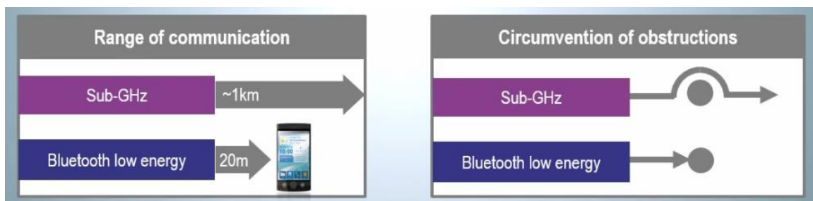
Figure 3. BLE and sub-GHz address different wireless connectivity requirements for IoT systems
